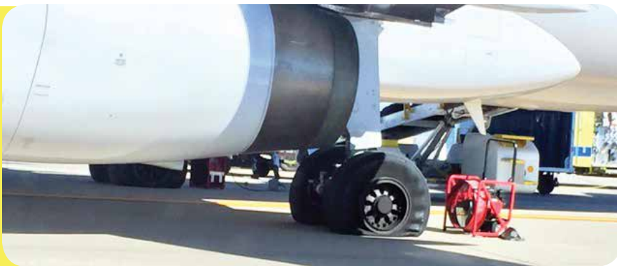
A popped tire was caused by the high-speed abort before takeoff
